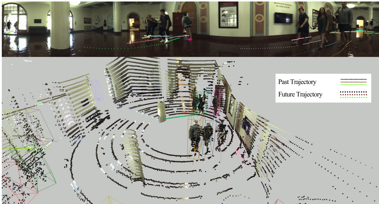
Figure 1: Trajectory Forecasting in JRDB-Traj dataset. The top figure displays the RGB image from the robot’s perspective, while the bottom figure shows the corresponding 3D point cloud. Solid lines indicate the observed past trajectories and dots represent the ground-truth future trajectories.
