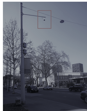
Figure 4: Thermal camera set-up: (a) the mounted four thermal cameras to capture traffic traversing (T1 – T4), (b) example of a overhead mounted thermal camera.
